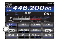
Touch [FWD] to switch the display screen, and then touch [TONE]. Rotate the MULTI knob to select the desired CTCSS Tone to be used. A total of 50 standard CTCSS tones are provided (see the CTCSS Tone Chart).
