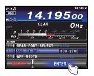
5. Press the **MENU(SETUP)** button or touch [**BACK**] on the TFT display to exit to normal operation.
