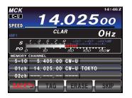
Rotate the MULTI knob to select a different memory channel. To exit from the Memory Check mode, press the A►M button momentarily once more.
