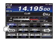
• The VOX (Voice Operated Xmit) circuit will engage the transmitter automatically when you speak into the microphone. For details of VOX operation refer to page 70.
