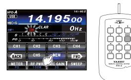
Touch [CH1] through [CH5] on the LCD or press any of the FH-2 keys numbered [1] through [5] to select that memory storage register.
