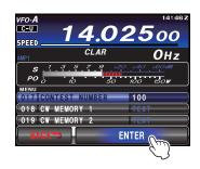
Press the MENU(SETUP) button or touch [BACK] on the LCD to exit to normal operation.
