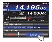
5. Press the **MENU(SETUP)** button or touch [**BACK**] on the LCD to exit to normal operation.
