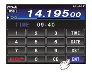
4. Touch [**DATE**] on the LCD to switch the screen.
