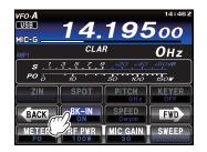
Touch [CH1] - [CH5] on the LCD or press the FH-2
