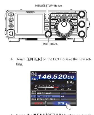
5. Press the **MENU(SETUP)** button or touch [**BACK**] on the LCD to exit to normal operation.
