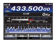
Press and hold in the microphone UP or DWN button for one second, or press the F(M-LIST) button followed by [SCAN] to start scanning in the specified direction on the VFO frequency.
