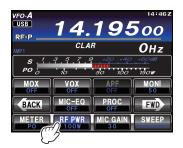
Adjust the microphone amplifier gain to match the microphone and your voice level: Touch [METER] on the LCD repeatedly to select the "ALC".
