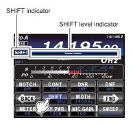
2. Rotate the **MULTI** knob to the left or right to reduce interfering signals.
