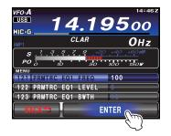
10. Press the **MENU(SETUP)** button or touch [**BACK**] on the LCD to return to normal operation. If you only touch [**BACK**] momentarily to exit the setup menu, none of the changes you performed will be stored.
