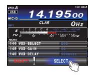
4) Rotate the **MULTI** knob while saying a brief syllable like "Ah" and listening to the hang time for the desired delay.
