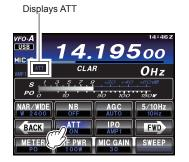
To restore full signal strength through the Attenuator circuit, touch [ATT] on the LCD to return the ATT display to the "OFF" position.
