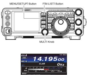
6) Press the **MENU(SETUP)** button or touch [**BACK**] on the LCD to exit to normal operation.
