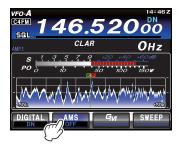
**VW (FR Mode)**: Digital voice data is transmitted using the entire 12.5 kHz bandwidth. High quality voice communication is possible.
