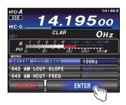
6. Press the **MENU** button or touch [**BACK**] on the LCD to exit to normal operation.
