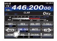
3. Touch [**TONE/DCS**] on the LCD repeatedly to select the desired CTCSS mode. If the repeater requires an uplink encoding tone, select "ENC." For both uplink and downlink encode/decode operation, choose "CTCSS". The available choices are:
