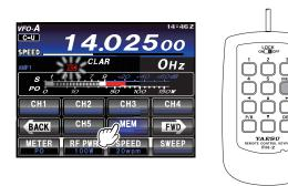
Touch [CH1] - [CH5] on the LCD or press an FH-2
