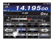
To adjust the Parametric Microphone Equalizer with the speech processor engaged, press the F(M-LIST) button, then touch [**PROC**] to select "ON".
