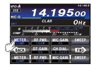
3. Press the **F(M-LIST)** button, then touch [**PROC**] to display the PROC level (from 1 to 100), confirming that the Speech Processor is engaged.
