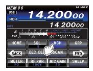
5. Rotate the **MULTI** knob to select the desired Memory Channel within the Selected Memory Group.
