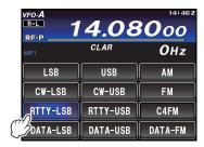
Press the MENU(SETUP) button. The Menu list will appear in the display. Rotate the MULTI knob to select Menu item "O60 PC KEYING". Touch [SE-LECT] on the LCD, then rotate the MULTI knob to set this Menu item to "RTS" or "DTR". Press the MENU(SETUP) button or touch [BACK] on the LCD to exit to normal operation.
