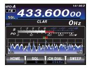
6. Press the **A**►**M** button. Make sure that the memory channel storing the receive frequency is selected.
