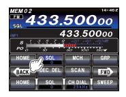
Press and hold in the microphone UP or DWN button for one second, or press the F(M-LIST) button followed by [SCAN] to start scanning in the specified direction.
