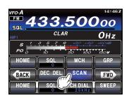
4. If the scanner halts on an incoming signal, the decimal point between the "MHz" and "kHz" digits of the frequency display will blink.
