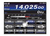
2. Rotate the **MULTI** knob to adjust the PITCH (300 Hz to 1,050 Hz).
