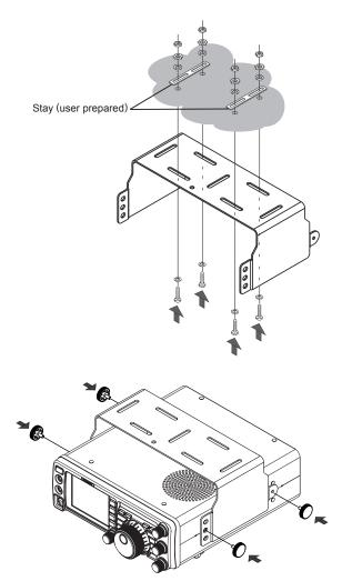
The viewing angle of the transceiver may be adjusted by changing the location of the front mounting screws.
