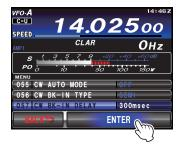
6. Press the **MENU(SETUP)** button or touch [**BACK**] on the LCD to exit to normal operation.
