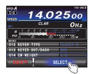
When your adjustments are complete, touch [EN-TER] on the LCD to save the new setting.
