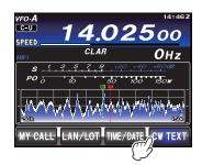
3. Rotate the **MULTI** knob to select the CW TEXT you want to input, then touch [**EDIT**]. The text input screen will appear.
