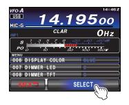
4. Touch **[ENTER]** on the LCD, then touch **[BACK]** on the LCD or press the **MENU** button to save the new setting and exit to normal operation.
