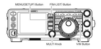
Rotate the MULTI knob to select the emergency channel ("EMG"), which is found between channels "5-10" and "01ch").
