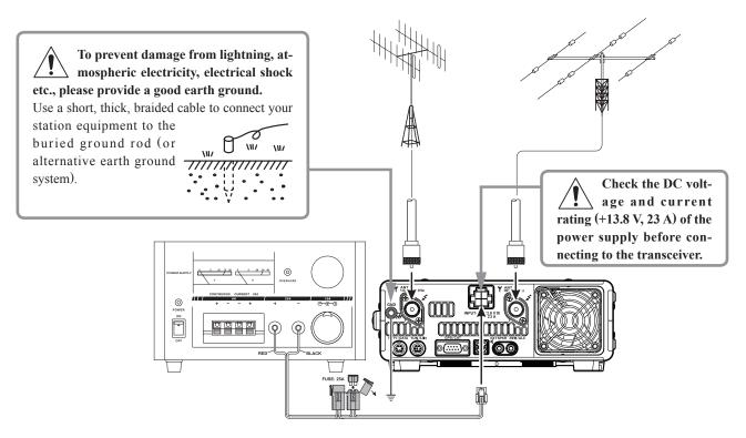
We recommend the use of the **FP-1030A** (USA market only) AC Power Supply. Other models of power supplies may be used with the **FT-991A**, but the 13.8 VDC input voltage, 23 Ampere current capability, and DC cable polarity guide-lines described above must be strictly followed.
