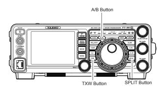
During Split operation, the VFO-A register will be used for reception, while the VFO-B register will be used for transmission. If you press the **SPLIT** button once more, Split operation will be cancelled.
