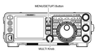
4. When the adjustment or setting is completed, touch [ENTER] on the LCD to save the new setting, then press the MENU(SETUP) button or touch [BACK] on the LCD to exit to normal operation.
