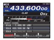
7. To register the transmit frequency, press and hold the **PTT** button on the microphone, and simultaneously press and hold the **A**► **M** button. A double beep will confirm that the **A**► **M** button was held in long enough and the data is registered. When the memory writing is completed, the receive frequency will be shown in the display.
