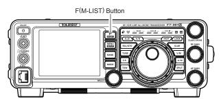
To disable the Digital NOTCH Filter, just repeat the above procedure, touching [**DNF**] on the LCD to choose "OFF". The "**DNF**" will turn off, confirming that the Digital NOTCH Filter is not active.
